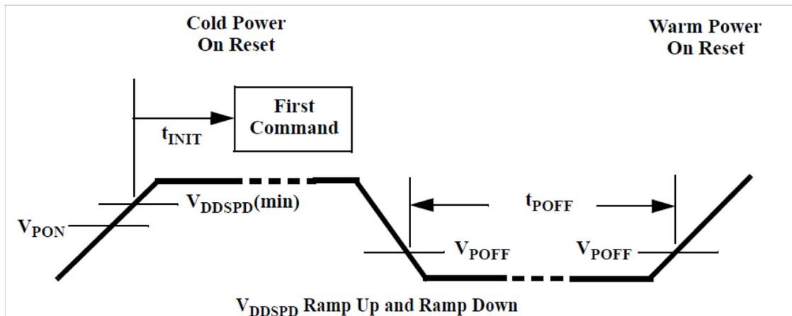
In order to prevent inadvertent Write operations during Power-up, a Power-On Reset (POR) circuit is included. On cold power on,  $V_{DDSPD}$  must rise monotonically between  $V_{PON}$  and  $V_{DDSPD(min)}$  without ringback to ensure proper startup. Once  $V_{DDSPD}$  has passed the  $V_{PON}$  threshold, the device is reset.
