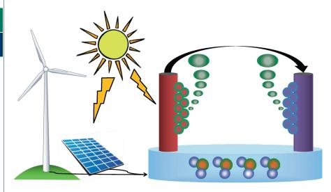
Schematic representation of the splitting of water via electrolysis, utilizing electricity,
